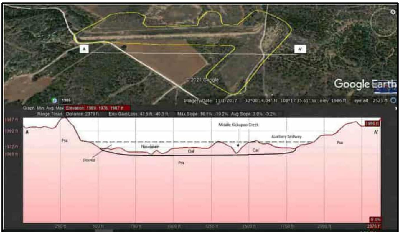
**Figure 73. Stratigraphic cross section of FRS No. 4 Study Area**
